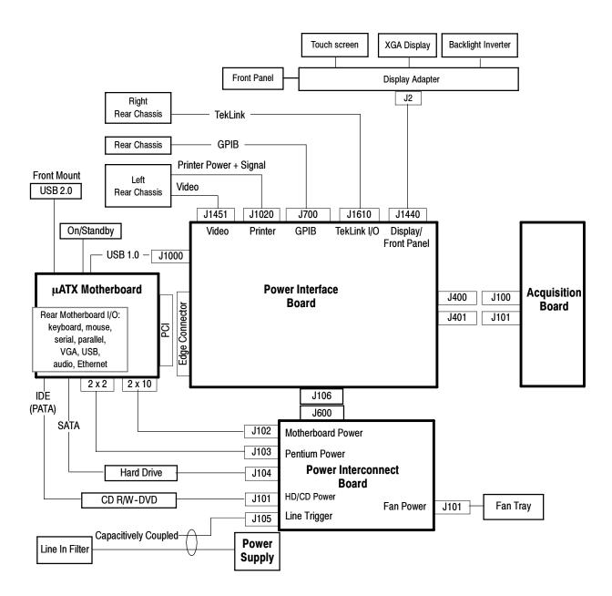
Figure 2-1: DPO7000 Series block diagram
