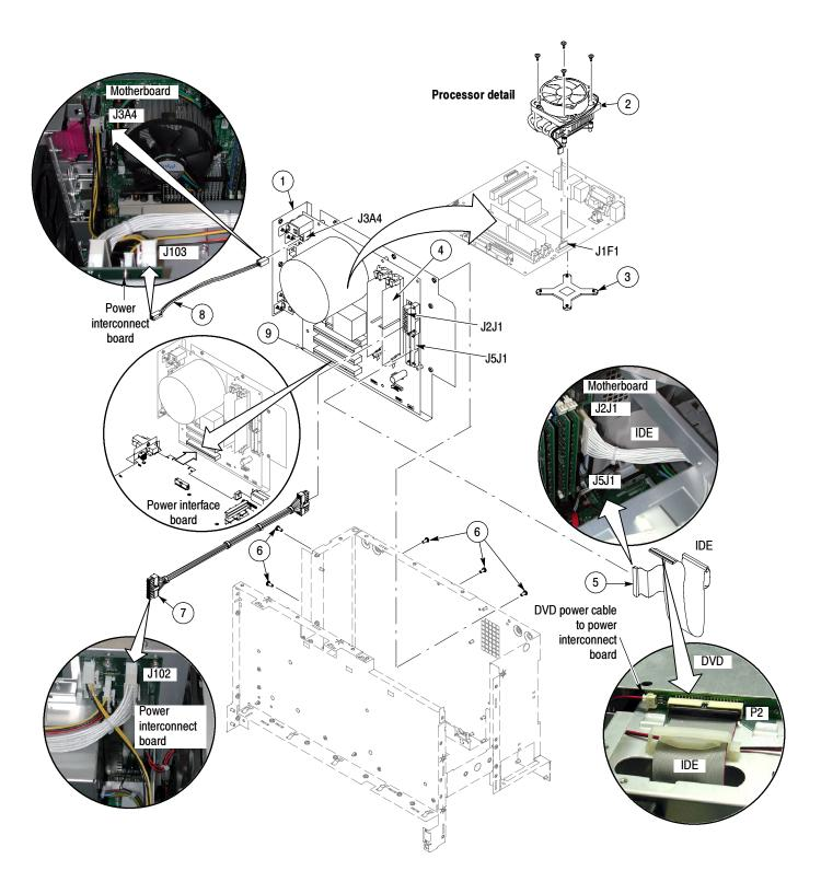
Figure 5-4: µATX Motherboard (<4.0 GHz models)
