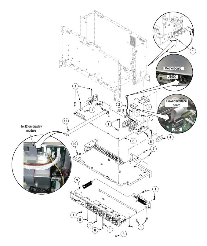
Figure 5-5: Power interface and Acquisition assemblies (<4.0 GHz models)
