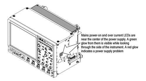
Figure 4-5: Location of power-on and over current LEDs
