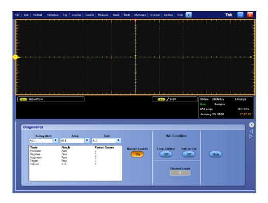
Figure 4-7: Diagnostics control panel
