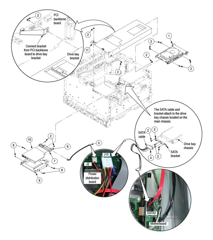
Figure 5-14: Drives ( $\geq$  4.0 GHz models)
