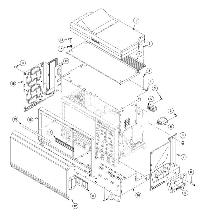
Figure 5-1: External parts (<4.0 GHz models)
