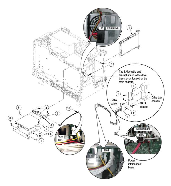
Figure 5-6: Drives (<4.0 GHz models)
