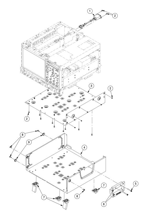
Figure 5-8: External parts 2 ( $\geq$  4.0 GHz models)
