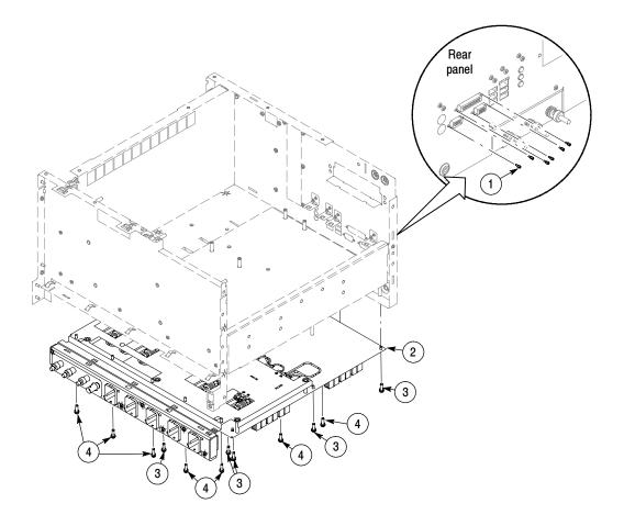
Figure 5-12: Acquisition assembly (  $\geq$  4.0 GHz models)
