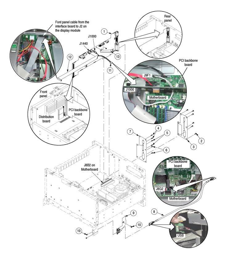
Figure 5-13: Interface board ( $\geq$  4.0 GHz models)
