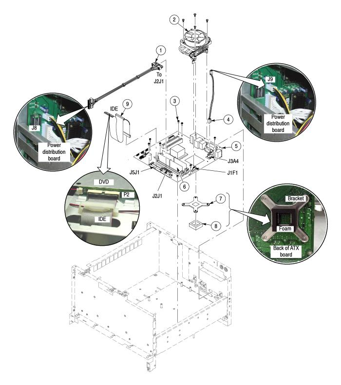
Figure 5-11: Atx assembly ( $\geq$  4.0 GHz models)
