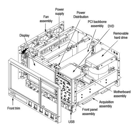
Figure 4-2: DPO70000 and DSA70000 Series module locations
